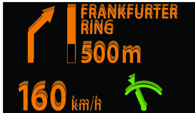
Example of "double image" from use of improper windshield
